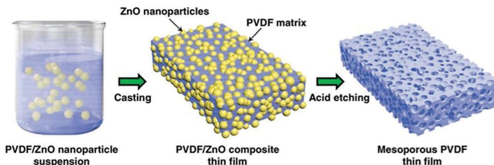
Fig. 8 Schematic of fabricating mesoporous piezoelectric PVDF thin films. Reproduced from ref. 147 with permission from John Wiley and Sons Ltd.
