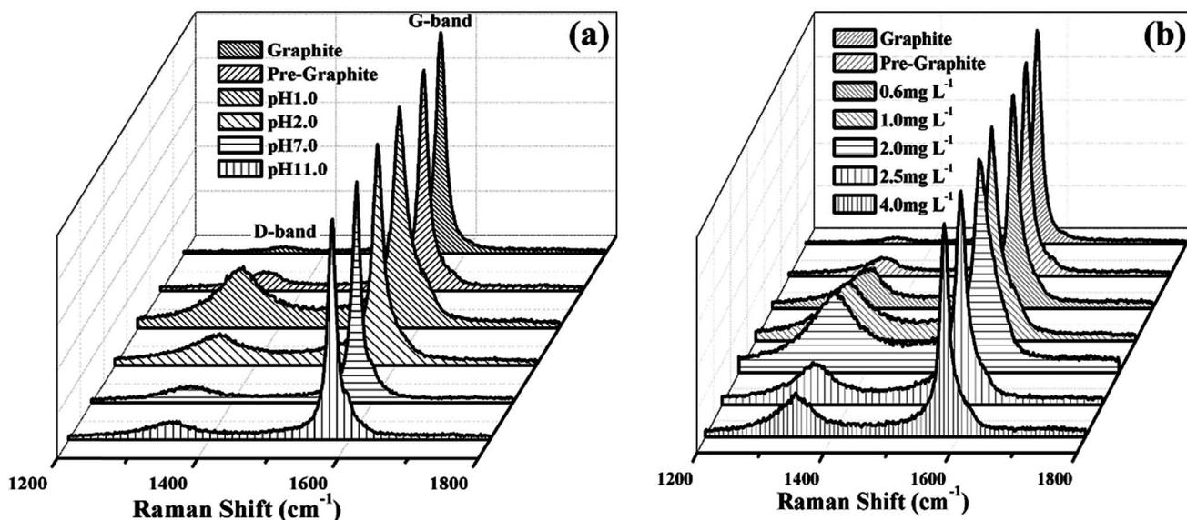
Fig. 2 Raman spectra of (a) as-received graphite, pre-graphite and pre-graphite samples treated with 1000  $\mu\text{g L}^{-1}$  Cr(vi) solution with different pH values ranging from 1.0 to 11.0 after treated with 30 min; and (b) pre-graphite samples treated with pH = 1.0 Cr(vi) solution with different initial Cr(vi) concentrations ranging from 600 to 4000  $\mu\text{g L}^{-1}$  Cr(vi) solution after treated with 30 min.
