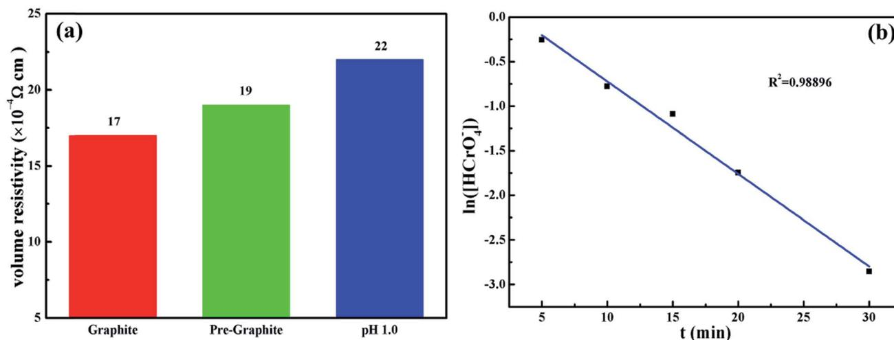
Fig. 4 (a) Volume resistivity of graphite, pre-graphite and pre-graphite after treated with  $1000 \mu\text{g L}^{-1}$  Cr(vi) with pH = 1.0 solution for 30 min; and (b) kinetic plot of  $\ln([\text{HCrO}_4^-])$  vs.  $t$  for 20.0 mg pre-graphite sample after treatment with 20.0 mL  $1000 \mu\text{g L}^{-1}$  Cr(vi) solution (pH = 1.0) under different treatment times at room temperature.
