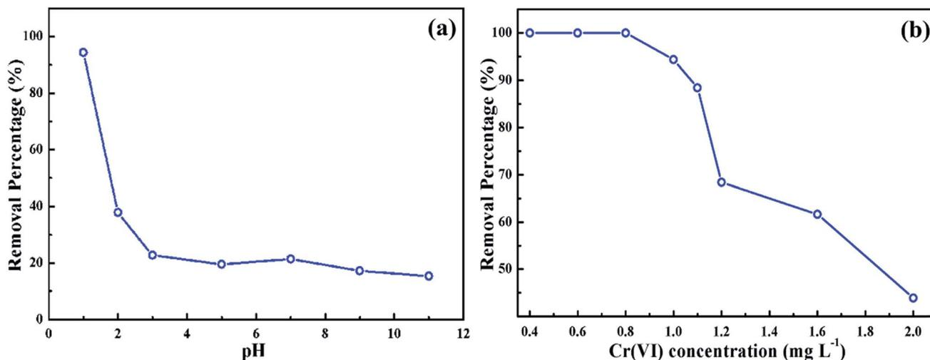
Fig. 1 Removal percentage of 20.0 mg pre-graphite for 20.0 mL Cr(vi) solutions with different (a) pH values after 30 min ultrasonic treatment at initial Cr(vi) concentrations of 1000  $\mu\text{g L}^{-1}$  at room temperature; (b) initial Cr(vi) concentrations after 30 min ultrasonic treatment at pH of 1.0 at room temperature.
