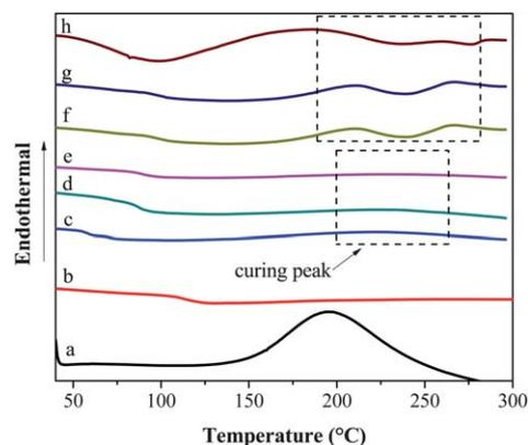
**Fig. 5** DSC curves of (a) the mixture of pure epoxy resin and curing agent, (b) cured pure epoxy and cured PNCs with (c) 1.0 wt% BaTiO<sub>3</sub> (500 nm), (d) 5.0 wt% BaTiO<sub>3</sub> (500 nm), (e) 10.0 wt% BaTiO<sub>3</sub> (500 nm), (f) 28.57 wt% BaTiO<sub>3</sub>-PANI (contains 10 wt% BaTiO<sub>3</sub> and 18.57 wt% PANI) and (g) 15.38 wt% BaTiO<sub>3</sub>-PANI (contains 5.38 wt% BaTiO<sub>3</sub> and 10 wt% PANI); (h) pure BaTiO<sub>3</sub>-PANI NPs.
