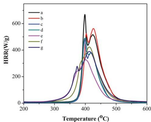
**Fig. 4** The HRR vs. temperature curves of (a) the cured pure epoxy and its PNCs with (b) 1.0 wt% BaTiO<sub>3</sub> (500 nm), (c) 10.0 wt% BaTiO<sub>3</sub> (500 nm), (d) 10.0 wt% BaTiO<sub>3</sub> (100 nm), (e) 28.57 wt% BaTiO<sub>3</sub>-PANI (contains 10 wt% BaTiO<sub>3</sub> and 18.57 wt% PANI) and (f) 15.38 wt% BaTiO<sub>3</sub>-PANI (contains 5.38 wt% BaTiO<sub>3</sub> and 10 wt% PANI), (g) 10.0 wt% PANI.
