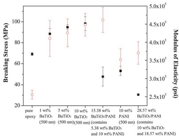
**Fig. 7** Breaking tensile stress (solid symbols) and modulus (open symbols) of elasticity of the cured pure epoxy and its PNCs.
