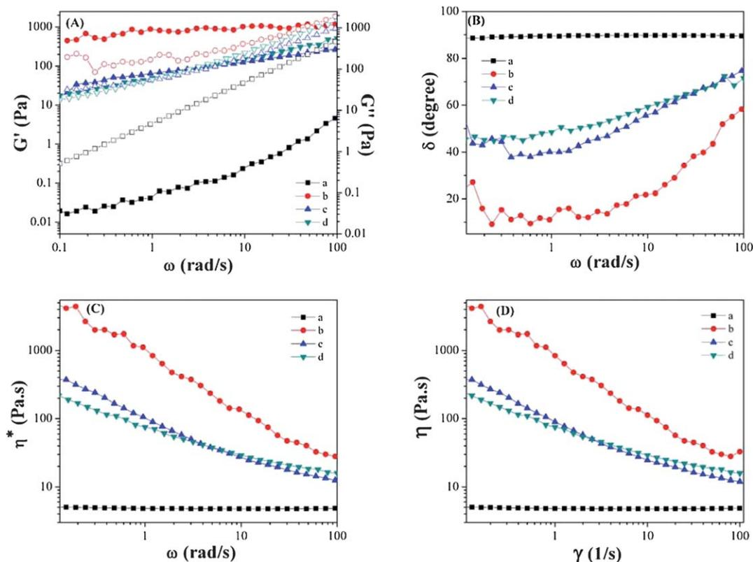
**Fig. 2** (A)  $G'$  and  $G''$  (solid and open symbols represent  $G'$  and  $G''$ , respectively), (B)  $\delta$ , (C) complex viscosity ( $\eta^*$ ) vs.  $\omega$ , and (D) viscosity vs. shear rate of the epoxy resin nanosuspensions with (a) 10.0 wt% BaTiO<sub>3</sub> (500 nm), (b) 28.57 wt% BaTiO<sub>3</sub>-PANI (contains 10 wt% BaTiO<sub>3</sub> and 18.57 wt% PANI), (c) 15.38 wt% BaTiO<sub>3</sub>-PANI (contains 5.38 wt% BaTiO<sub>3</sub> and 10 wt% PANI) and (d) 10.0 wt% PANI.
