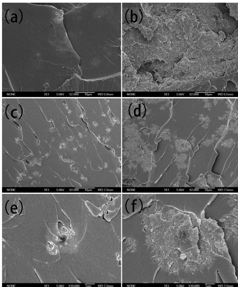
**Fig. 8** SEM images of the fracture surface of (a) the cured pure epoxy, and the PNCs with (b) 10.0 wt% PANI NPs, (c and e) 10.0 wt% BaTiO<sub>3</sub> NPs (500 nm), and (d and f) 28.57 wt% BaTiO<sub>3</sub>-PANI (contains 10 wt% BaTiO<sub>3</sub> and 18.57 wt% PANI).
