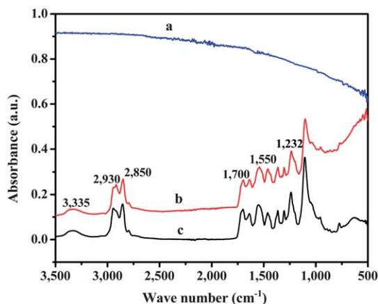
**Fig. 2** FT-IR spectra of the (a) MWNTs, (b) MWNT-PU composites, and (c) pure PU films.
