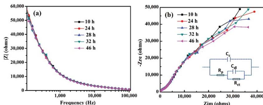
**Fig. 7** EIS of the MWNT/PU-SS electrode. Inset is the equivalent circuit.
