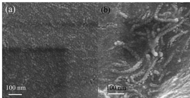
**Fig. 1** SEM microstructures of the (a) pure PU and (b) MWNT-PU composite film from a cross-sectional view.
