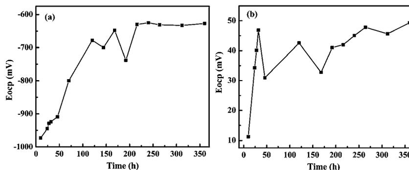
Fig. 5 The open circuit potential ( $E_{ocp}$ )–time curves for (a) SS and (b) MWNT/PU-SS in 3.0 wt% NaCl solution.
