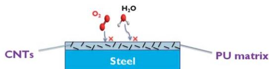
**Scheme 4** Illustration of the anticorrosion mechanism of MWNT-PU composite coating.
