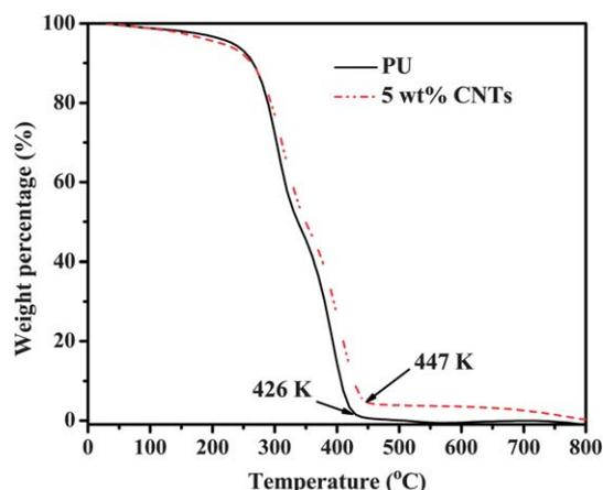
**Fig. 3** TGA of the pure PU and the MWNT-PU nanocomposites.
