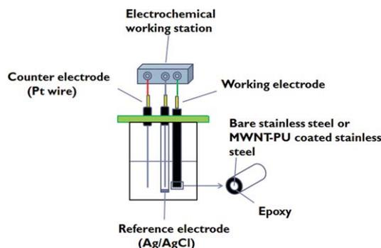
**Scheme 3** Experimental configuration for the corrosion test.
