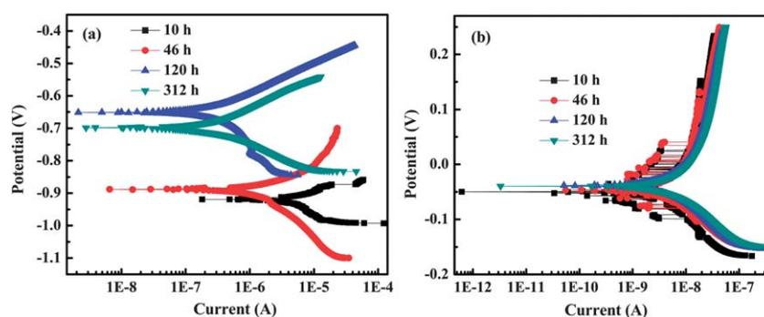
Fig. 6 Tafel curves of the (a) SS and (b) MWNT/PU-SS electrodes.
