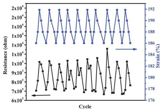
Fig. 4 *In situ* resistance of the MWNT-PU composite thin films in response to cyclic strain.
