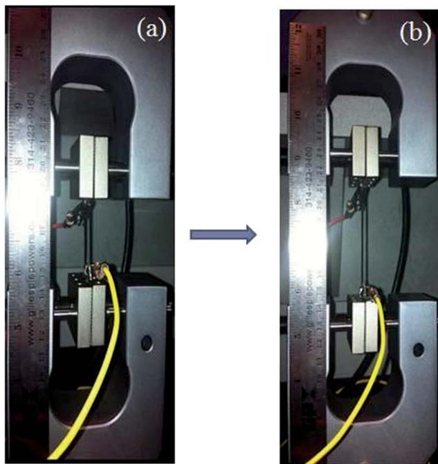
**Scheme 2** Illustration of the experimental set up for *in situ* electrical conductivity measurement during the cyclic strain test. (a) and (b) show the composite film at different elongations during the stretching process.
