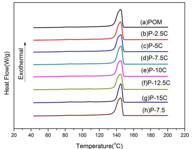
FIG. 6. DSC curves of (a) POM, (b) P-2.5C, (c) P-5C, (d) P-7.5C, (e) P-10C, (f) P-12.5C, (g) P-15C, and (h) P-7.5. [Color figure can be viewed at wileyonlinelibrary.com]
