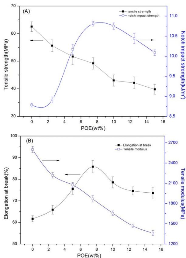
FIG. 2. (A) Tensile strength and Notch impact strength (B) Elongation at break and Tensile modulus vs POE (wt%) of POM and compatibilized POM/POE/GMA-g-HDPE (Note: when POE (wt%) was 0, the material was POM). [Color figure can be viewed at wileyonlinelibrary.com]
