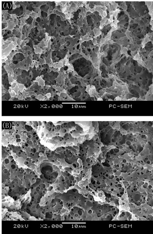
FIG. 3. Tensile fracture surface of (A) P-7.5C and (B) P-7.5.
