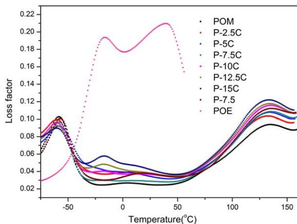
FIG. 9. Loss factor vs temperature of POM, modified POM blends and POE. [Color figure can be viewed at wileyonlinelibrary.com]
