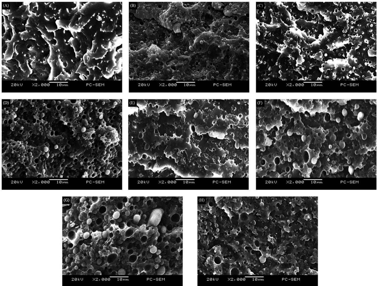
FIG. 1. SEM micrographs of the cryo-fractured surface of (A) POM; (B) P-2.5C; (C) P-5C; (D) P-7.5C; (E) P-10C; (F) P-12.5C; (G) P-15C; and (H) P-7.5.
