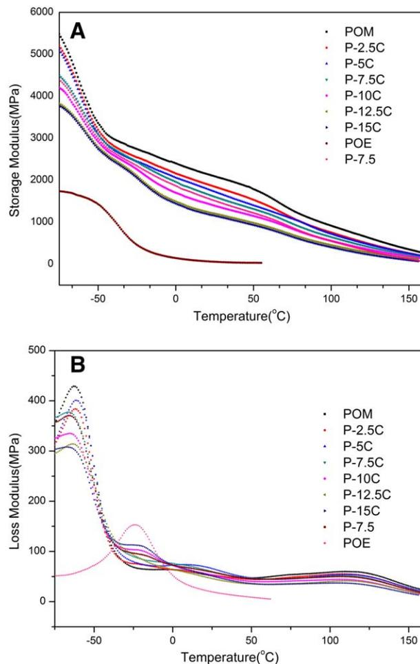
FIG. 8. (A) Storage modulus; and (B) Loss modulus of POM, modified POM blends and POE. [Color figure can be viewed at wileyonlinelibrary.com]
