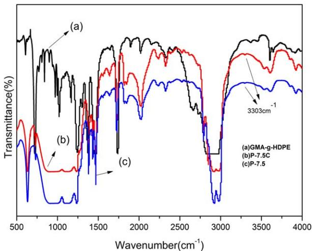
FIG. 4. FTIR spectra of (a) GMA-g-HDPE, (b) P-7.5C, and (c) P-7.5. [Color figure can be viewed at wileyonlinelibrary.com]
