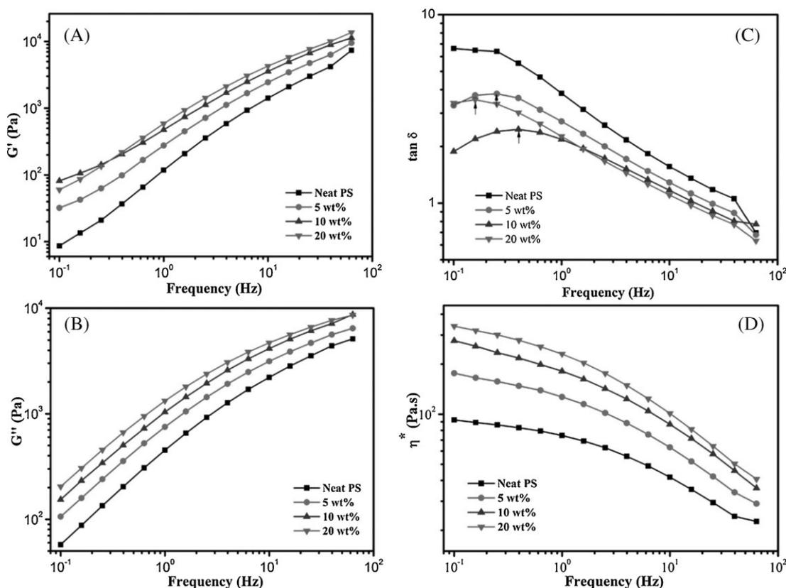
Figure 8. A) Storage modulus ( $G'$ ), B) loss modulus ( $G''$ ), C) mechanical loss factor ( $\tan\delta$ ), and D) complex viscosity ( $\eta^*$ ) as a function of frequency for PS and its PNCs.
