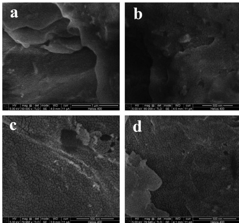
Figure 1. SEM images of the (a) pure PS and the PNCs with a particle loading of (b) 5 wt%, (c) 10 wt%, and (d) 20 wt%, respectively.
