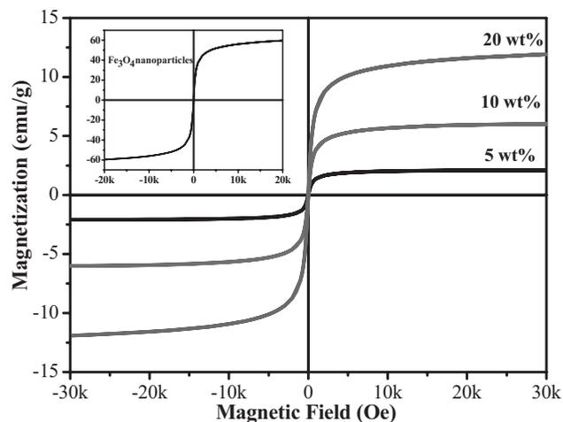
Figure 9. Room temperature hysteresis loops of PS/ $\text{Fe}_3\text{O}_4$  nanocomposites with a particle loading of 5, 10, and 20 wt%, respectively; insert shows pure NPs.
