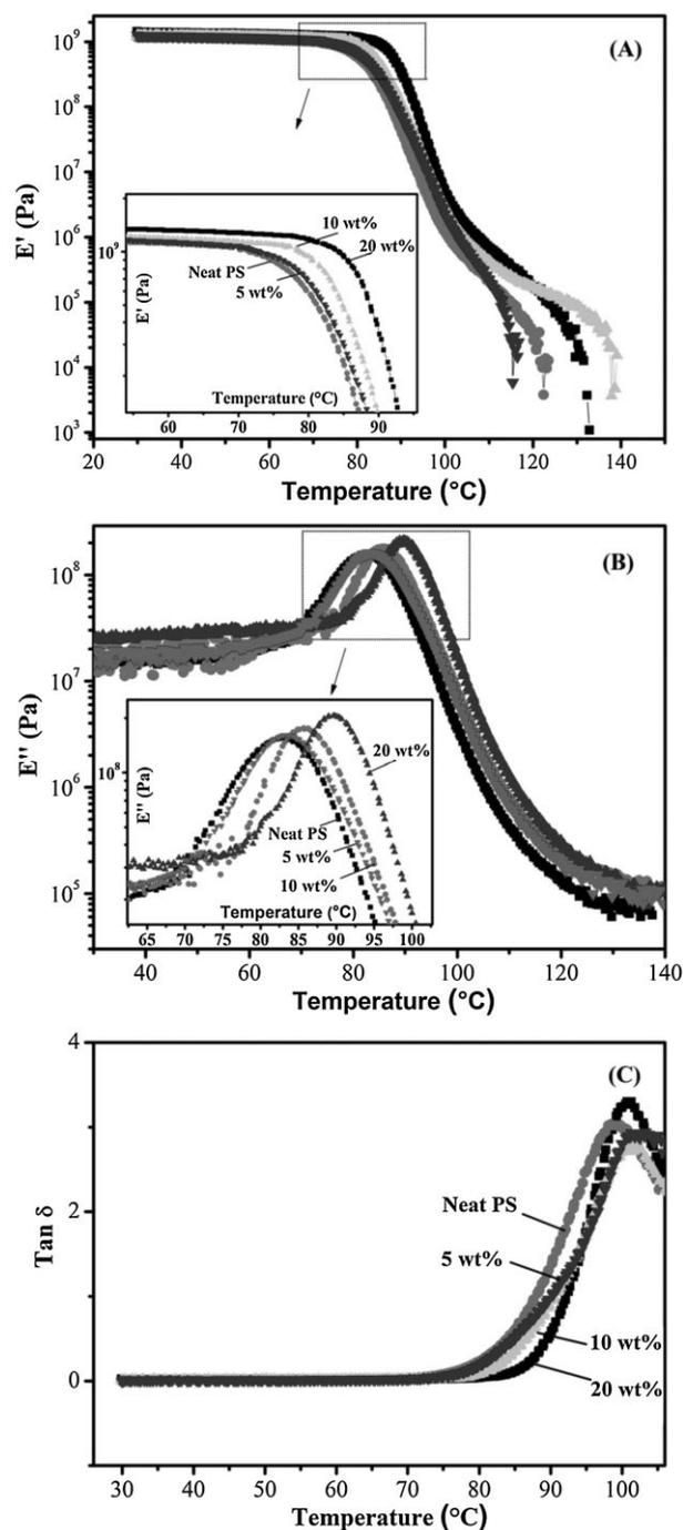
Figure 7. A) Storage modulus ( $E'$ ), B) loss modulus ( $E''$ ), and C)  $\tan\delta$  versus temperature for the neat PS and its nanocomposites with different Fe<sub>3</sub>O<sub>4</sub> nanoparticle loadings.
