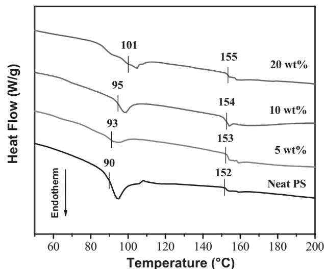
Figure 5. DSC thermograms of pure PS and PS/ $\text{Fe}_3\text{O}_4$  nanocomposites with different  $\text{Fe}_3\text{O}_4$  nanoparticle loadings.
