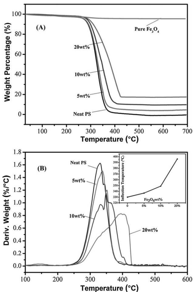
Figure 4. A) TGA weight loss curves and B) derivative weight loss curves of pure PS, Fe<sub>3</sub>O<sub>4</sub> and PS/Fe<sub>3</sub>O<sub>4</sub> PNCs. Inserted: the inflection point as a function of the loading of Fe<sub>3</sub>O<sub>4</sub> NPs.
