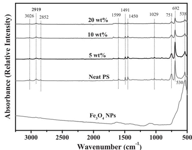
Figure 3. FT-IR spectra of pure PS and its PS/Fe<sub>3</sub>O<sub>4</sub> nanocomposites.
