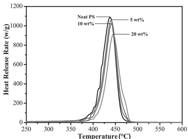
Figure 6. The HRR curves of PS/Fe<sub>3</sub>O<sub>4</sub> nanocomposites with a particle loading of 5, 10, and 20 wt%, respectively.
