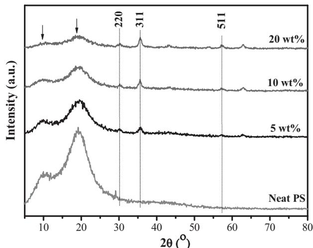
Figure 2. XRD patterns of pure PS and PS/Fe<sub>3</sub>O<sub>4</sub> nanocomposites.
