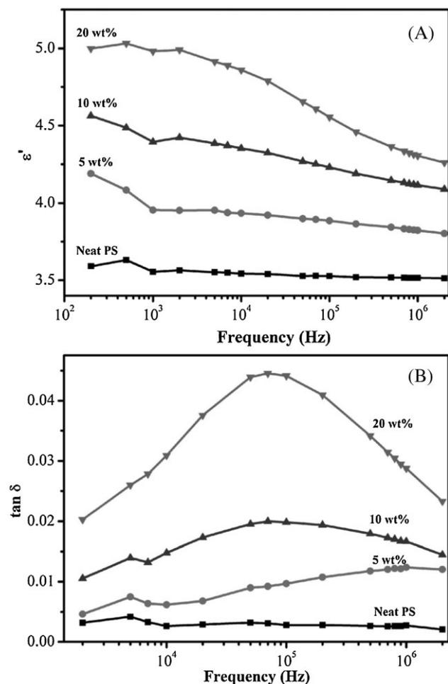
Figure 10. A) Real permittivity, B) dielectric loss tangent as a function of frequency for neat PS and its PNCs with different nanoparticle loadings.
