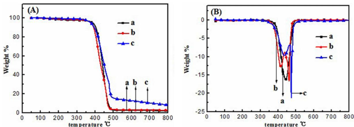
**Figure 1.** (a) TGA and (b) DTG curves of the PA66 system, (a') pure PA66, (b') PA66/14%AlPi composites, and (c') PA66/10%AlPi/1% nano-silica composites. TGA: thermogravimetric analysis; AlPi: aluminum diethylphosphinate; PA66: polyamide 66; DTG: derivative thermogravimetry.
