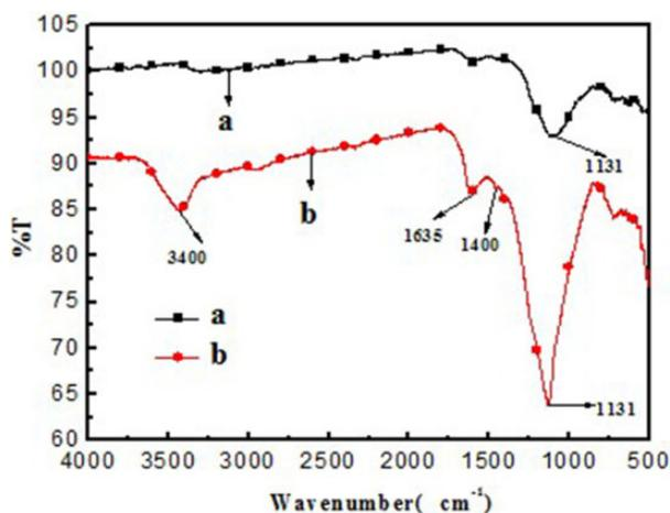
**Figure 3.** The FTIR spectrum of (a) the PA66/14%AlPi composites and (b) the PA66/10%AlPi/1% nano-silica composites after CONE test. AlPi: aluminum diethylphosphinate; PA66: polyamide 66; CONE: cone calorimeter; FTIR: Fourier transform infrared spectrometer.
