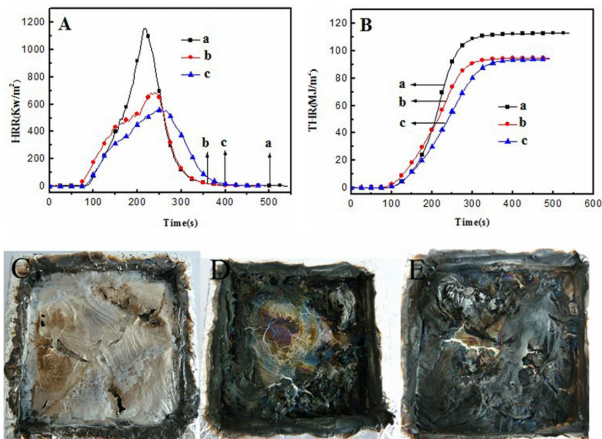
**Figure 2.** (a) HRR curves, (b) THR curves of (a') pure PA66, (b') PA66/14%AlPi composites, and (c') PA66/10%AlPi/1% nano-silica composites, and (c), (d), and (e) digital photos of the residues after CONE test for pure PA66, PA66/14%AlPi composites and PA66/10%AlPi/1% nano-silica composites. AlPi: aluminum diethylphosphinate; PA66: polyamide 66; HRR: heat release rate; CONE: cone calorimeter; THR: total heat release.
