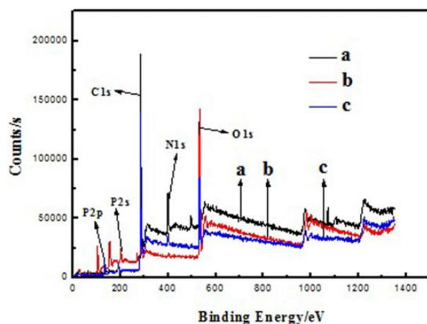
**Figure 5.** The XPS of (a) pure PA66, (b) the PA66/14%AlPi composites, and (c) the PA66/10%AlPi/1% nano-silica composites char residue after CONE test. AlPi: aluminum diethylphosphinate; PA66: polyamide 66; CONE: cone calorimeter; XPS: X-ray photoelectron spectroscopy.
