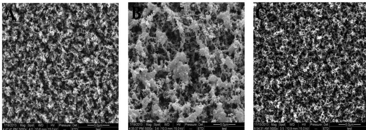
**Figure 4.** The SEM photographs of (a) pure PA66, (b) the PA66/14%AlPi composites, and (c) the PA66/10%AlPi/1% nano-silica composites after CONE test (5000 $\times$ ). AlPi: aluminum diethylphosphinate; PA66: polyamide 66; CONE: cone calorimeter; SEM: scanning electron microscopy.
