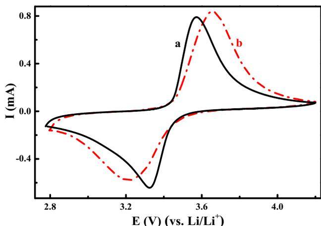
Fig. 5. CV curves of (a) OP-LiFePO<sub>4</sub>/MWNTs and (b) S-LiFePO<sub>4</sub>/C samples.
