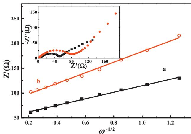
Fig. 9.  $Z'$  as a function of  $\omega^{-1/2}$  of (a) OP-LiFePO<sub>4</sub>/MWNTs and (b) S-LiFePO<sub>4</sub>/C samples at low frequency range. Inset shows the Nyquist plots of (a) OP-LiFePO<sub>4</sub>/MWNTs and (b) S-LiFePO<sub>4</sub>/C samples.
