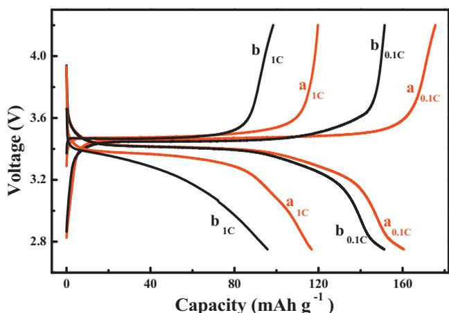
Fig. 6. Charge and discharge curves of the battery cell (a) OP-LiFePO<sub>4</sub>/MWNTs and (b) S-LiFePO<sub>4</sub>/C samples at different rates.
