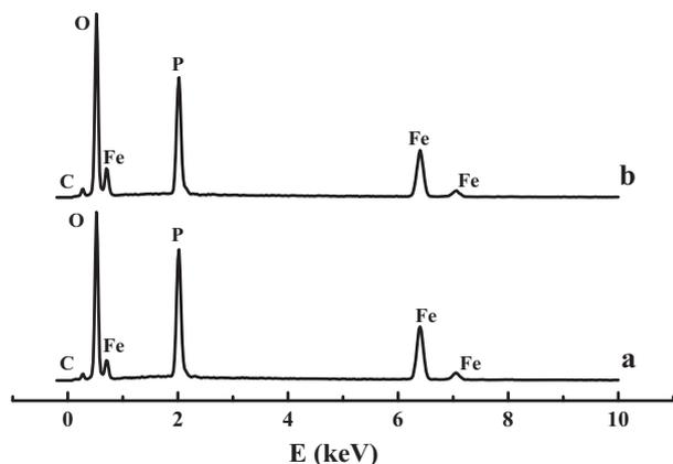
Fig. 2. EDX spectra of (a) OP-LiFePO<sub>4</sub>/MWNTs and (b) S-LiFePO<sub>4</sub>/C samples.
