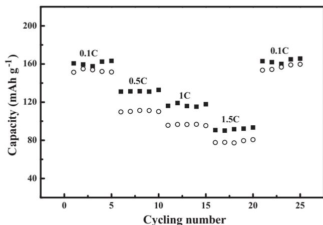
Fig. 8. Cycling performance of the discharge capacity for the battery cell (a) OP-LiFePO<sub>4</sub>/MWNTs and (b) S-LiFePO<sub>4</sub>/C samples at different rates.
