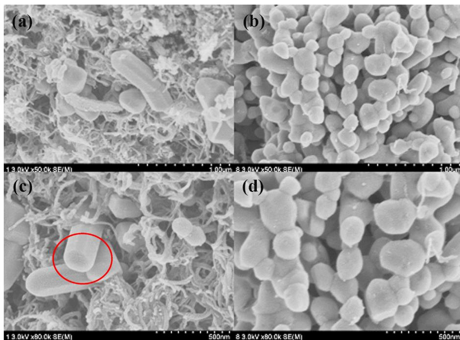
Fig. 4. SEM images of (a) OP-LiFePO<sub>4</sub>/MWNTs, and (b) S-LiFePO<sub>4</sub>/C samples; Enlarged SEM images of (c) OP-LiFePO<sub>4</sub>/MWNTs, and (d) S-LiFePO<sub>4</sub>/C samples.
