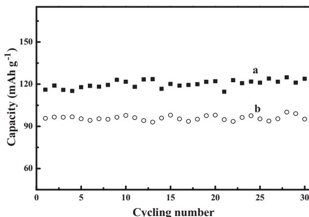
Fig. 7. Cycling performance of the discharge capacity for the cell (a) OP-LiFePO<sub>4</sub>/MWNTs and (b) S-LiFePO<sub>4</sub>/C samples at rate of 1C.
