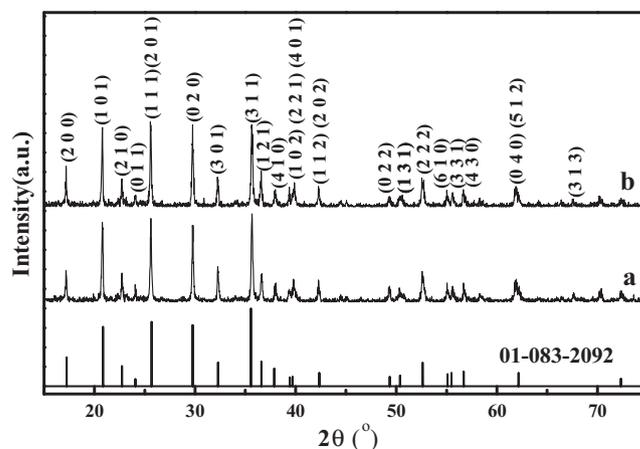
Fig. 3. XRD patterns of (a) OP-LiFePO<sub>4</sub>/MWNTs and (b) S-LiFePO<sub>4</sub>/C samples.
